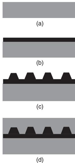
**Figure 3.19** The main steps in the formation of self-assembled quantum dots: (a) initial surface, (b) deposition of the two-dimensional wetting layer, (c) formation of three-dimensional islands once the critical thickness for the 2D to 3D growth transition is reached and (d) overgrowth of the dots
