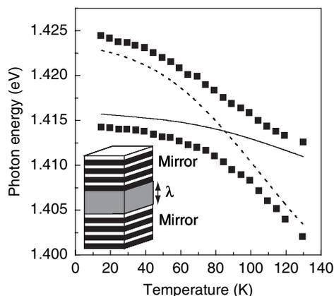
**Figure 3.51** Solid symbols show the temperature dependence of the energies of the quantum well exciton and cavity mode (photon) of a GaAs–AlGaAs microcavity, which exhibit an anti-crossing around 90 K. The lines show the calculated exciton (dashed line) and cavity (solid line) energies in the absence of coupling. The inset shows the physical structure of the microcavity. Data courtesy of Adam Armitage, University of Sheffield
