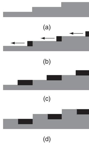
**Figure 3.16** The growth of quantum wires on a vicinal surface: (a) initial stepped surface, (b) initial growth of the wire semiconductor in the corners of the steps, (c) growth proceeds outwards along the steps and (d) second half of step completed with growth of the barrier semiconductor. The figure greatly exaggerates the angle of the surface
