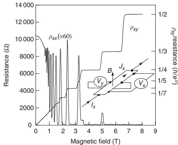
**Figure 3.26** The integer quantum Hall effect as measured for a 2DEG in a GaAs–AlGaAs single heterojunction at a temperature of 50 mK. The inset shows the experimental geometry used for Hall effect measurements. Data reproduced from M. A. Paalanen, D. C. Tsui and A. C. Gossard, *Phys. Rev. B* **25**, 5566 (1982). Copyright 1982 by the American Physical Society
