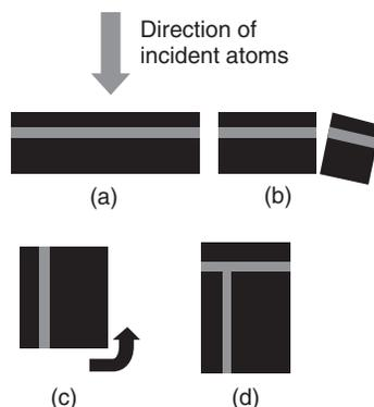
**Figure 3.15** The growth sequence used to produce cleaved edge overgrowth quantum wires: (a) growth of initial quantum well, (b) in situ cleaving, (c) rotation of the structure and (d) growth of a second quantum well on the cleaved surface
