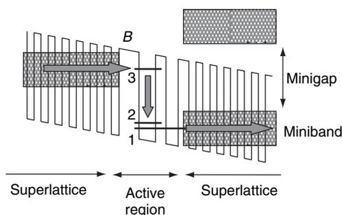
**Figure 3.47** The band structure of a quantum cascade laser. Electrons are transported between stages via the miniband of a superlattice, before tunnelling through barrier B into the upper lasing state, state 3. The minigap formed between the minibands of the superlattice prevents electrons tunnelling directly out of state 3. Courtesy of John Cockburn, University of Sheffield
