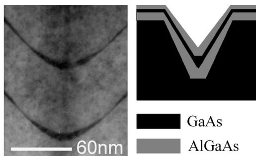
**Figure 3.18** A schematic cross section of a V-groove quantum wire and a transmission electron microscope image of two stacked GaAs–AlGaAs quantum wires. Image courtesy of Dr Gerald Williams, QinetiQ, Malvern
