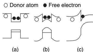
**Figure 3.24** (a) n-type modulation doping of a quantum well showing the transfer of electrons from the barriers to the well; (b) the band edge profile of a modulation-doped quantum well, including the effects of band bending which results from the non-zero space charges in the well and barriers; (c) the production of a 2DEG in a modulation-doped single heterojunction
