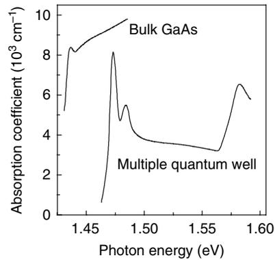
**Figure 3.34** Comparison of the room temperature absorption spectra of bulk GaAs and a 77-period GaAs–Al<sub>0.28</sub>Ga<sub>0.72</sub>As multiple quantum well with 10 nm wide wells. Data reproduced by permission of the American Institute of Physics from D. A. B. Miller, D. S. Chemla, D. J. Eilenberger, P. W. Smith, A. C. Gossard and W. T. Tsang, *Appl. Phys. Lett.* **41**, 679 (1982)
