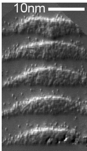
**Figure 3.23** An STM cross-sectional image of the cleaved surface of a structure containing five layers of InAs self-assembled quantum dots with 10 nm thick intermediate GaAs layers. The thin GaAs layers result in a vertical alignment of the quantum dots. Reproduced by permission of the American Institute of Physics from D. M. Bruls, P. M. Koenraad, H. W. M. Salemink, J. H. Wolter, M. Hopkinson and M. S. Skolnick, *Appl. Phys. Lett.* **82**, 3758 (2003)
