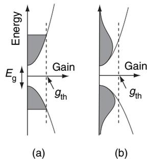
**Figure 3.44** Electron and hole distributions in the conduction and valence bands of a bulk semiconductor laser at (a) absolute zero temperature and (b) non-zero temperature. In (b) thermal excitation of carriers to higher energy states has reduced the maximum gain below the value,  $g_{th}$ , required for laser action
