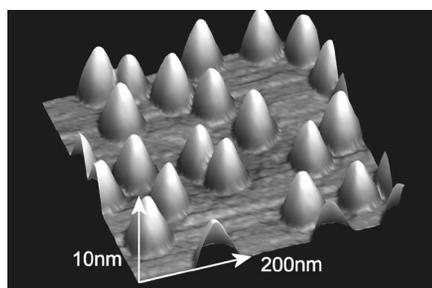
**Figure 3.21** An AFM image of uncapped InAs self-assembled quantum dots grown on a GaAs substrate. Note the different horizontal and vertical scales. Image courtesy of Mark Hopkinson, University of Sheffield
