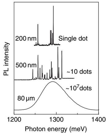
**Figure 3.22** PL spectra of different numbers of self-assembled quantum dots recorded through holes of different sizes formed in an opaque metal mask. For small numbers of dots the sharp emission lines due to individual dots are observed. Data courtesy of Jonathan Finley, University of Sheffield
