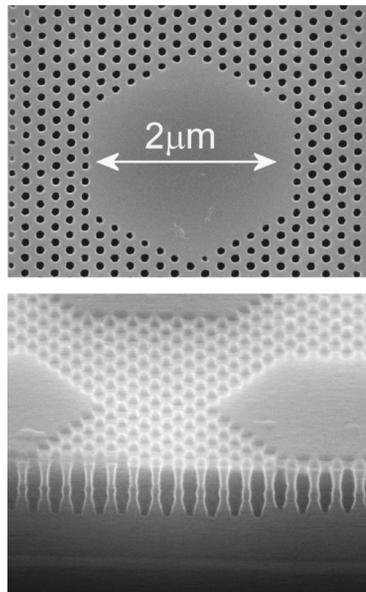
**Figure 3.52** Two-dimensional photonic structure consisting of periodic arrays of holes and a series of unpatterned regions which act as ultra-small cavities within which photons are confined by the surrounding photonic structure. The upper image is recorded via the upper surface of the structure, the lower image is of a cleaved edge. Data courtesy of Alan Bristow, University of Sheffield
