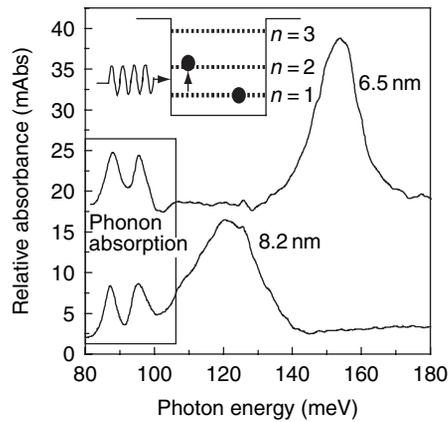
**Figure 3.35** Intraband absorption spectra of two 50-period GaAs multiple quantum well structures with wells of width 6.5 and 8.2 nm. Transitions between the  $n = 1$  and  $n = 2$  confined electron levels. The inset shows a schematic diagram of the absorption process. Data reproduced by permission of the American Institute of Physics from L. C. West and S. J. Eglash, *Appl. Phys. Lett.* **46**, 1156 (1985)
