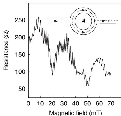
**Figure 3.32** The Aharonov–Bohm effect in a 1.8  $\mu\text{m}$  diameter ring, measured at a temperature of 280 mK. The inset shows the geometry of the structure. Data and figure reproduced from G. Timp, P. M. Mankiewich, P. deVegvar, R. Behringer, J. E. Cunningham, R. E. Howard, H. U. Baranger and J. K. Jain, *Phys. Rev. B* **39**, 6227 (1989). Copyright 1989 by the American Physical Society
