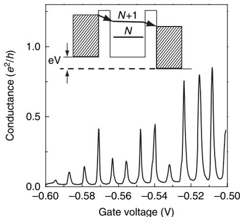
**Figure 3.30** Coulomb blockade oscillations for an electrostatically defined quantum dot measured at a temperature of 10 mK. The inset shows the transport of a single electron through the structure. Data reproduced from L. P. Kouwenhoven, N. C. van der Vaart, A. T. Johnson, W. Kool, C. J. P. M. Harmans, J. G. Williamson, A. A. M. Staring and C. T. Foxon, *Zeitschrift für Physik B* **85**, 367 (1991). Copyright 1991 Springer-Verlag
