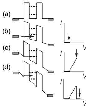
**Figure 3.27** Schematic conduction band diagram of a double-barrier resonant tunnelling structure. The band structure is shown for different applied voltages and with the corresponding current: (a) no applied voltage, (b) voltage below the first resonance, (c) in resonance with the lowest energy state in the quantum well, and (d) above the first resonance
